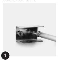
Fix clips with suitable screws (min 3 clips per metre or every 500mm/20").
